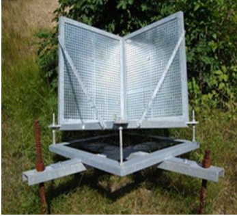
A corner reflector installed in the Idro landslide area
